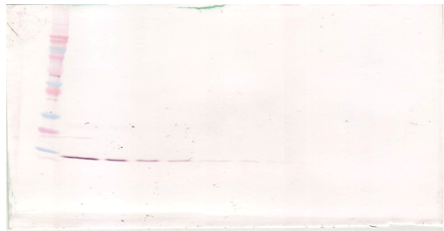
ARG56588 anti-IL4 antibody [1.3_4F11-2G3] WB image Western blot: 250 - 0.24 ng (left to right) of Human IL-4 stained with ARG56588 anti-IL4 antibody [1.3_4F11-2G3], under non-reducing conditions.
