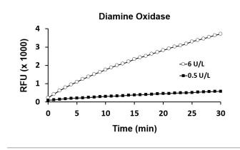
ARG82249 Diamine Oxidase Assay Kit (Fluorometric) enzyme kinetics graph
